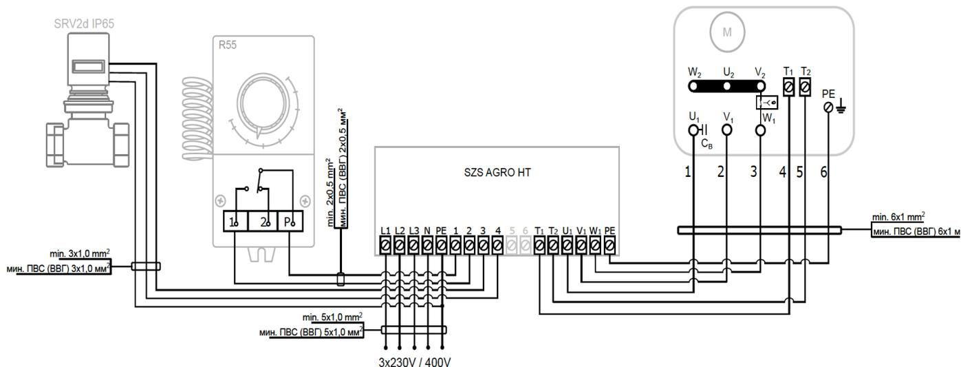
R55 thermostat controls the valve (SRV2d IP65 - optional) and the fan. SZS AGRO HT Cabinet cooperates with thermal protection mounted inside the fan, indicates the operating status or failures, controls the phase order, phase asymmetry and phase loss. The cabinet is equipped with a function to change the fan rotation (LEFT / RIGHT).
