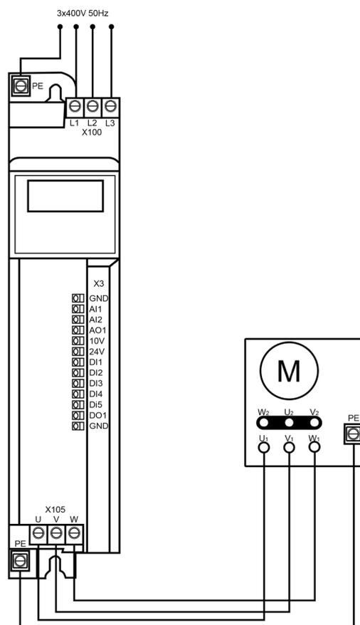
Inverter- (FAL 0.75 3x400) enables stepless adjustment of fan speed using a signal from the microclimate computer (not provided by FLOWAIR). The inverter has the ability to connect the thermal protection of the fan and change fan rotation LEFT / RIGHT.
