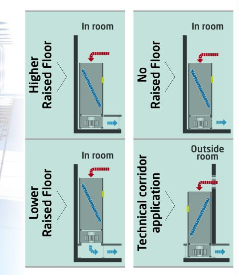
The chilled water coil that extends across the whole width of the cabinet allows to maximize the heat exchange, and to contain the pressure losses aeraulic.
