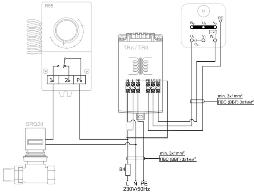
Thermostat R55 controls the operation of SRV2d valve. TRd speed regulator allows for 5-step fan air flow switch.
