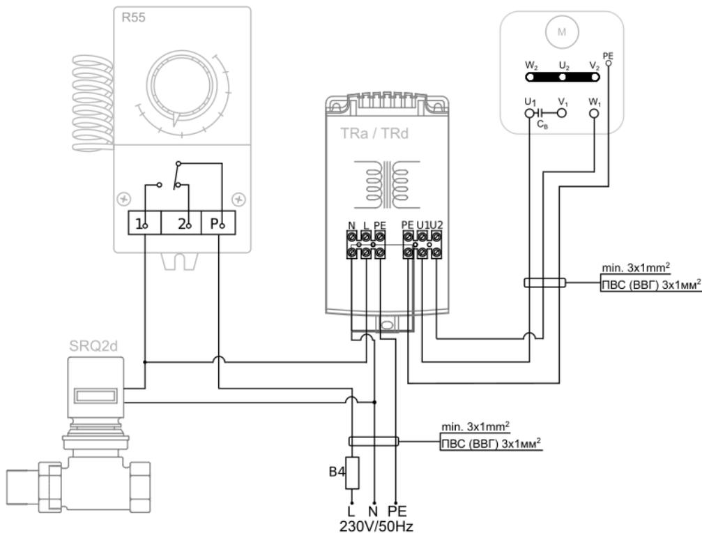
Thermostat R55 controls the operation of SRV2d valve and TRd speed regulator. TRd allows for 5-step fan air flow switch.
